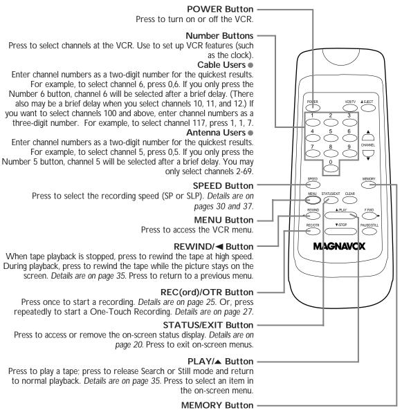
Press to memorize a tape position at which the real-time counter was set to 0:00:00. Details are on page 34.
